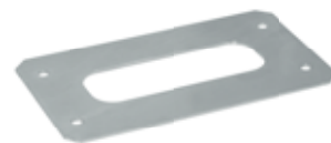
Foundation plate with anchor bolts included. Motor and floor fixing distance 269 mm x 106 mm, no. 4 Ø 12 mm.
